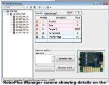
RoboPlus Manager screen showing details on the seven AX-12 servos.
