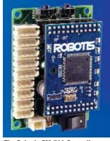
The Robotis CM-700 Controller with sub-board attached.
